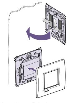
2. install the control using the supplied double-sided tape
