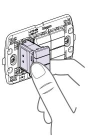
2. remove the control from its enclosure
